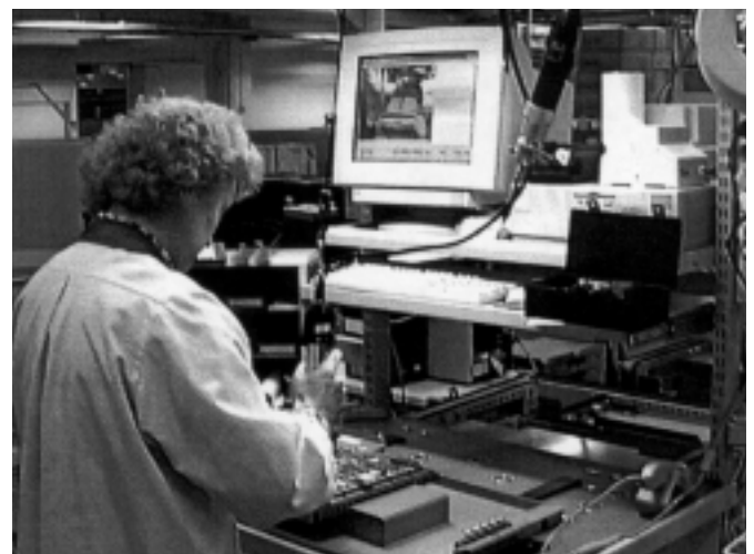
Figure 2. An interactive task support system supports the end assembly of a GSM base station in the Nokia Networks Oulu plant. Picture courtesy of Nokia Networks.
